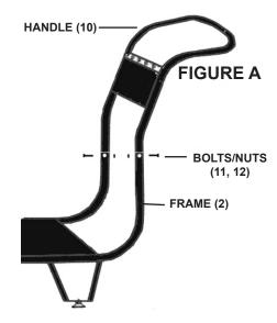
2. To attach the Handle (10) to the Frame (2), insert the lower portion of the Handle into the Frame. Then secure the Handle to the Frame, using two Bolts and two Nuts. (See Figure A.)
